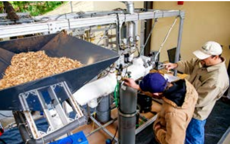
TOP: Wood chips derived from forest biomass are a promising source of renewable energy. BOTTOM: SERC engineers (left to right) Kyle Palmer and Greg Chapman work with a torrefier that converts forest waste into energy-dense material which can replace coal in power plants.
