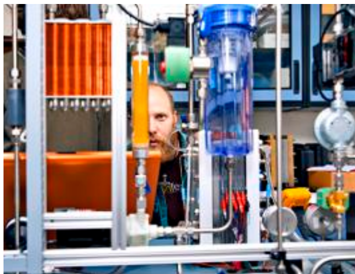
HSU senior engineering student, River Hume, works with the H 2 E 3 fuel cell test station as part of his Advanced Thermodynamics lab.
